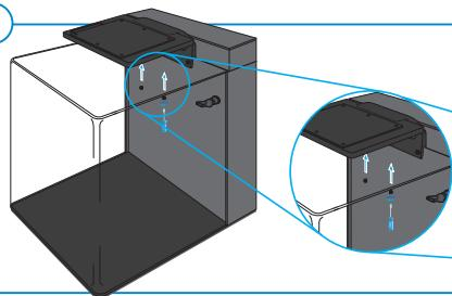
Secure the lighting with the mounting screws (13) using the screwdriver (14).
