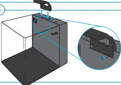
Place the lighting fixture (4) on the edge of the sump and hand tighten the mounting screws for the fixture (12) so that it can be moved even when the sump cover is placed.
