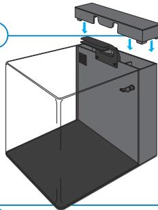
Place the cover (17) on the sump. Adjust the position of the lighting fixture so it fits in the openings of the cover, then tighten the screws.
